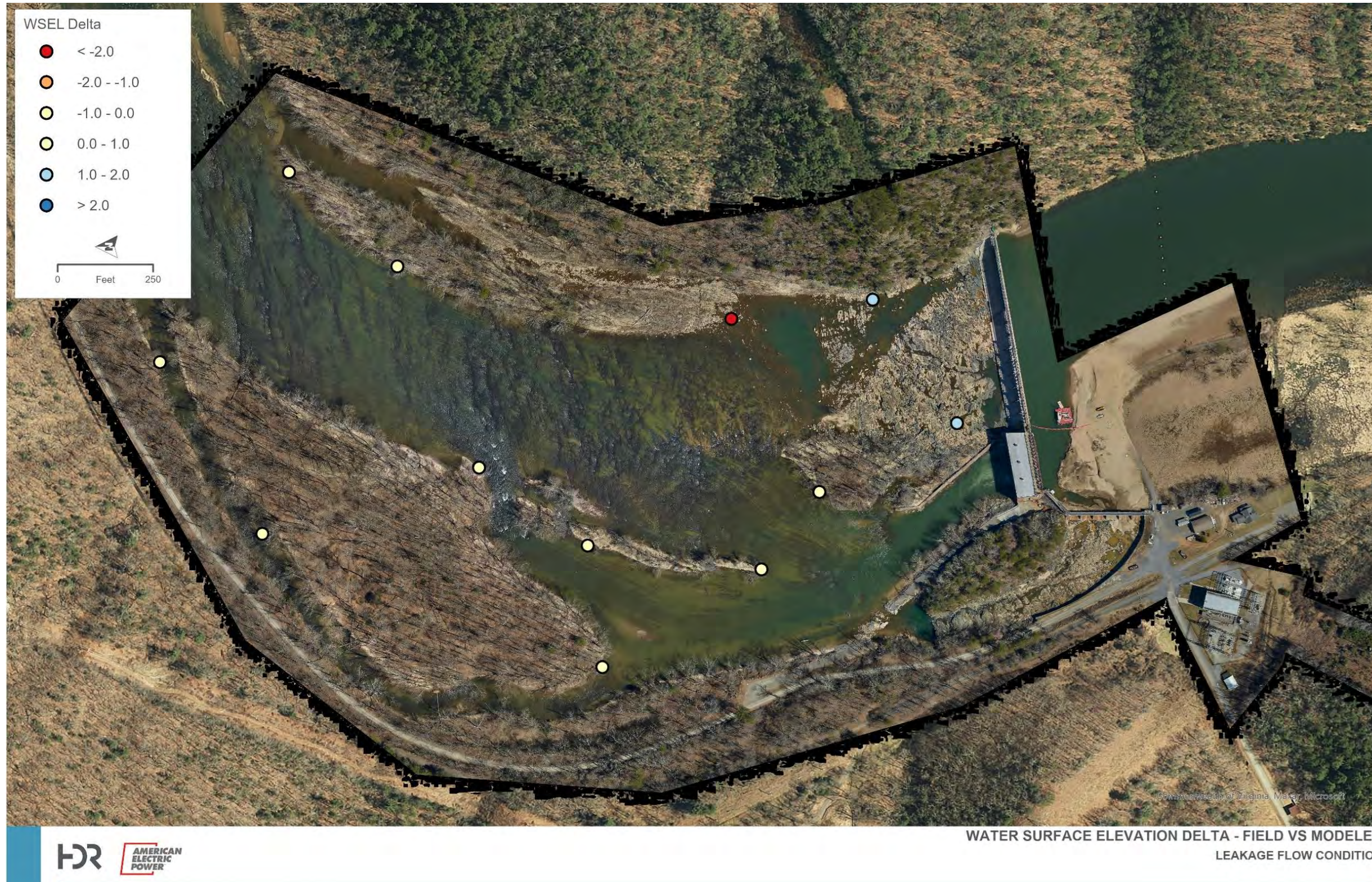
Figure 4-1. Field vs Modeled Water Surface Elevations – Leakage Flow
