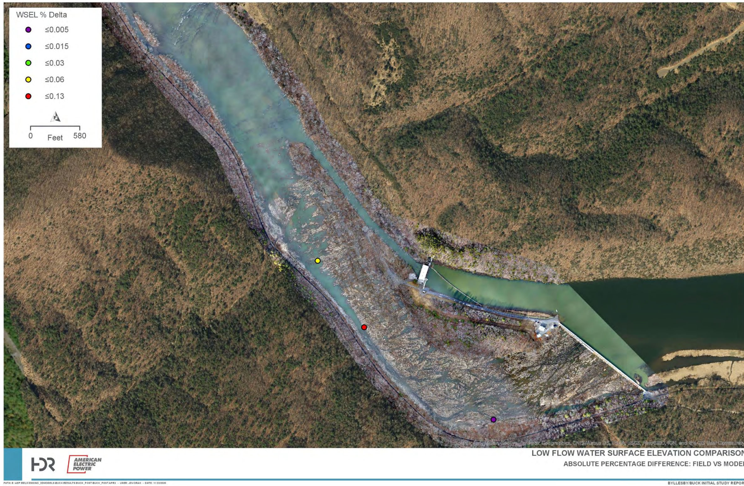
Figure 4-2. Field vs Modeled Water Surface Elevations – Day 2 (Low) Target Flow
